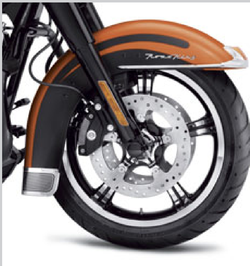
B. ANARCHY 5-SPOKE WHEEL – 18" CONTRAST CHROME (SHOWN WITH RAW OPEN FLOATING BRAKE ROTORS)
